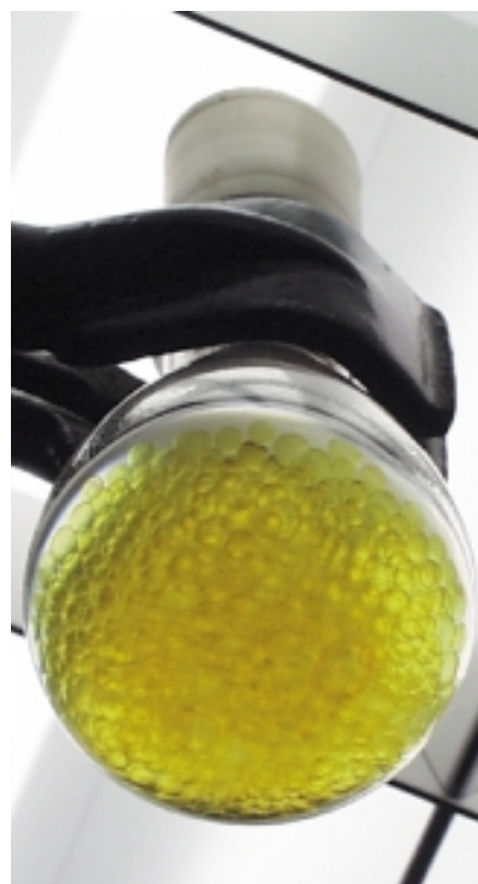
Figure 3. Round-bottomed flask containing a suspension of polymer beads p\mathbf{17}\cdot\text{AlMe} (diameter > 1000 \mu\text{m} ) in toluene.
