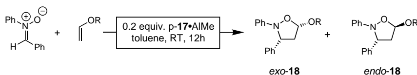
Scheme 11. 1,3-Dipolar cycloaddition of diphenyl nitron to vinyl ethers to give cycloadducts 18 , mediated by BINOL copolymers p\mathbf{17}\cdot\text{AlMe} . R = Et or t Bu.
